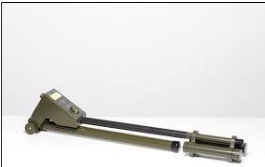
Afb.4 – Passieve magnetometer Sensys type SBL-10.
