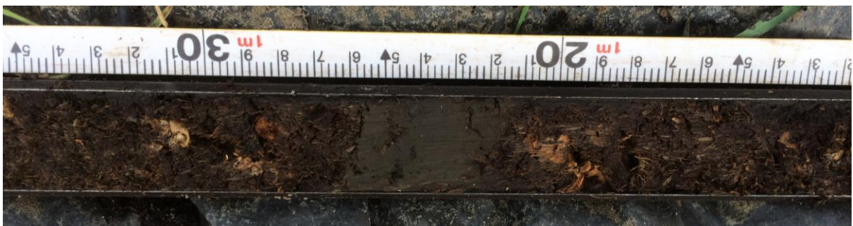
Boring 2: klei-inschakeling in rietveenpakket (Hollandveen laagpakket)
