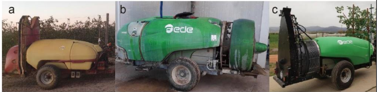
Fig. 1 Three air-assisted spraying systems used for the field trials: a) Hardy tower sprayer, b) Fede axial-fan sprayer, c) Fede tower sprayer.
