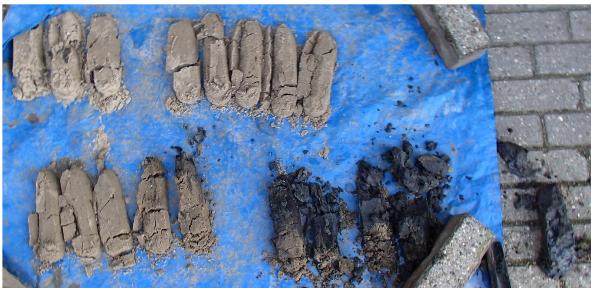
Boring 1: 10 – 210 cm –Mv. De bovenste 10 cm was bestrating. De zwarte grond is vervuild.
