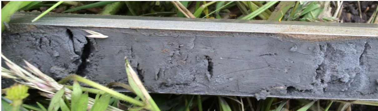
Boring 2: detail kleiige inschakeling
