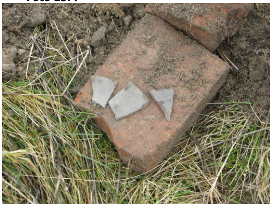
Asbest in grond A1 (gat 05 / boring 07)
