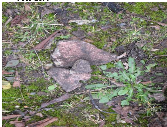
Asbest in grond A2 (gat 11 / boring 14)
