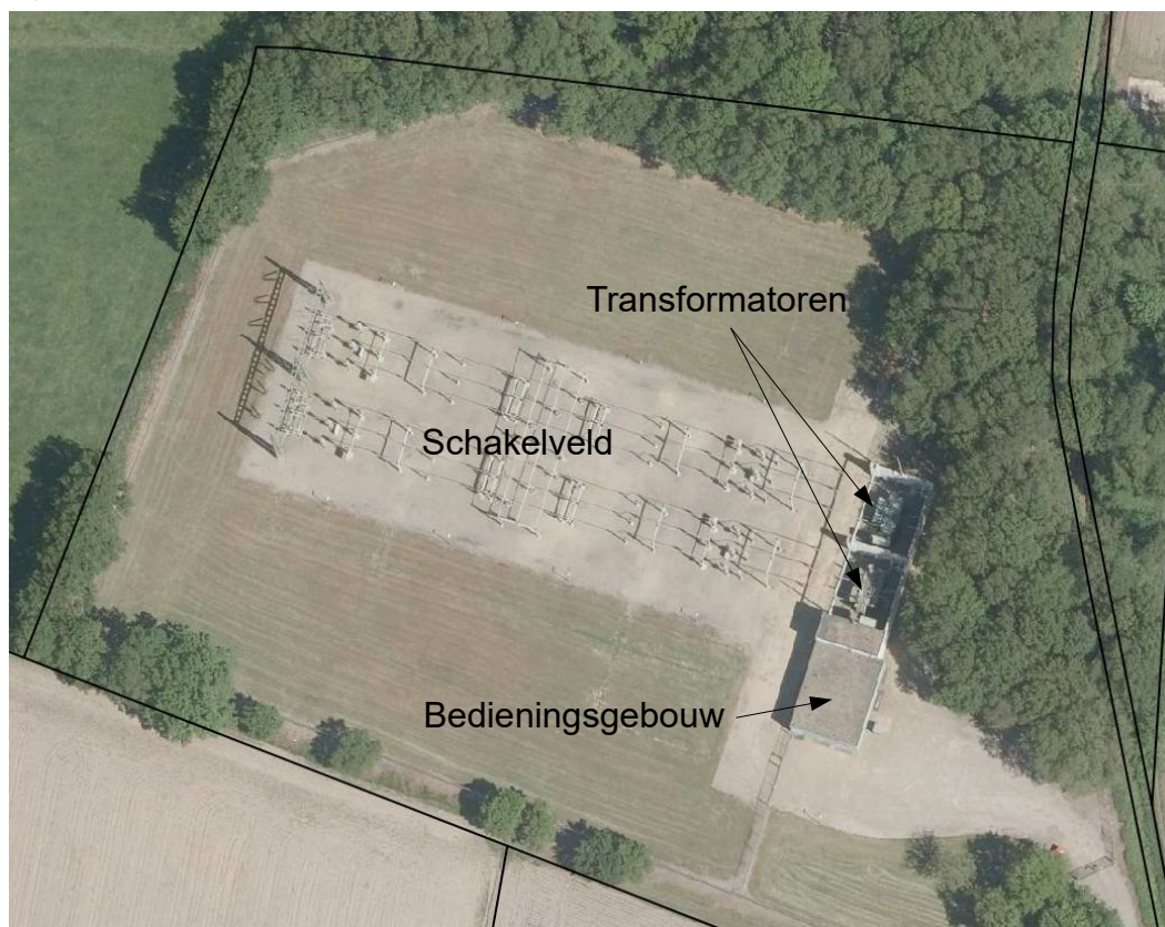
f2.1 Lay-out 150 kV station Kelpen-Oler
