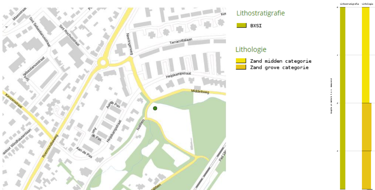
Figuur 5: Geologisch profiel boring te Steyl (boring B58E1009, bron Dinoloket, TNO)
