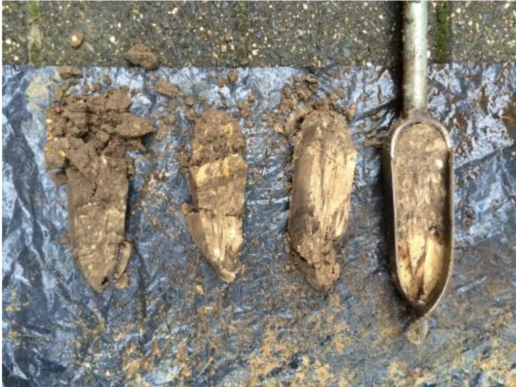
Boring 4: Detail boorkernen.
