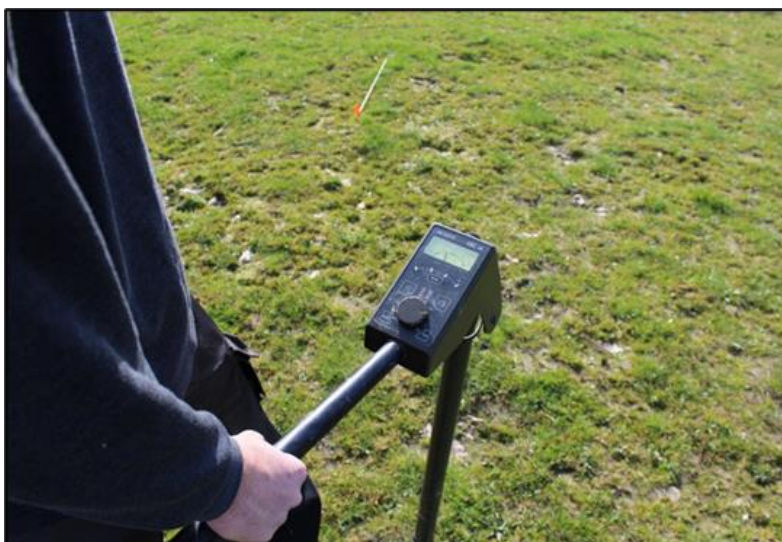
Afb.2 – Passieve magnetometer Sensys SBL-10.
