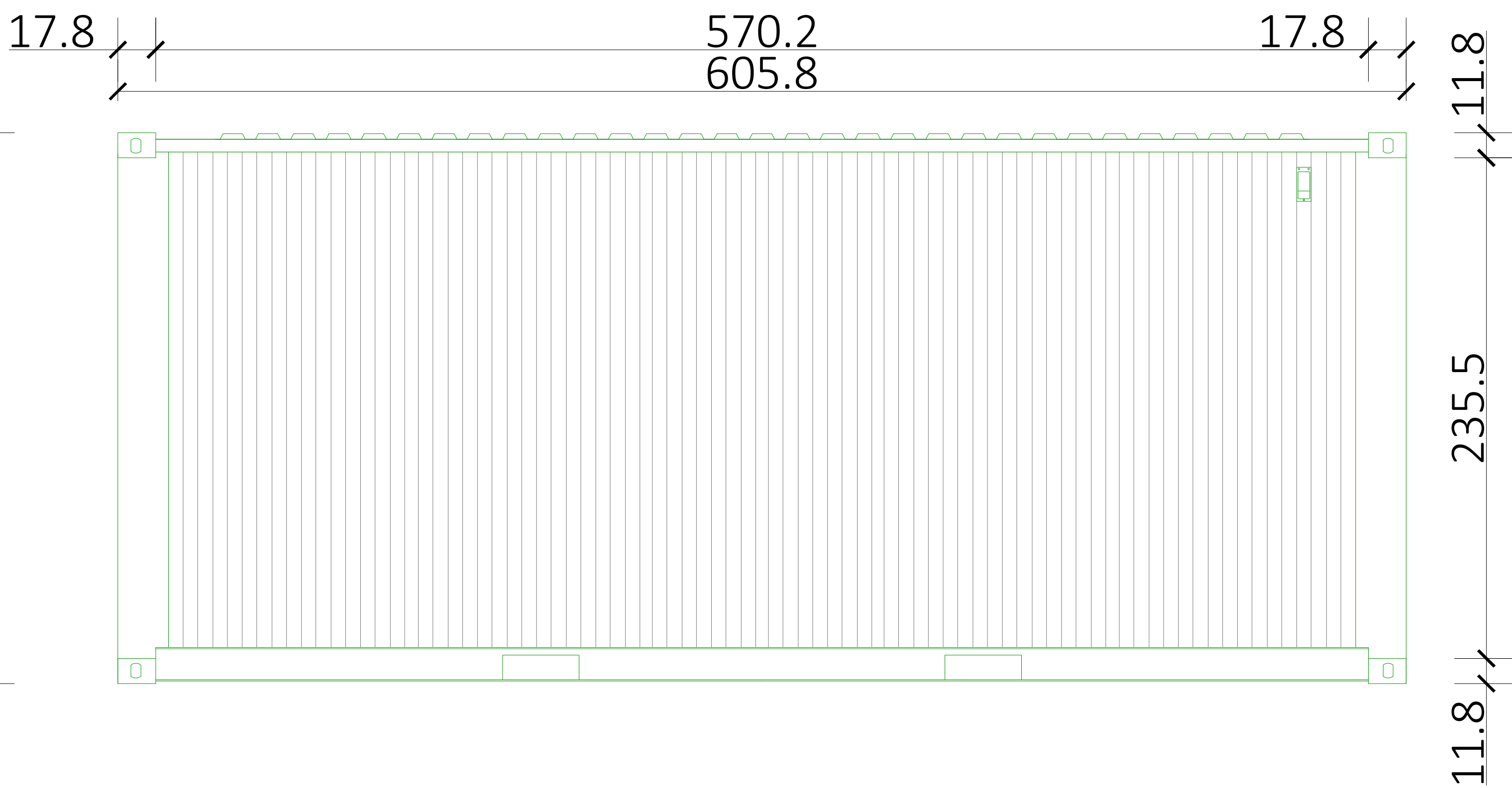
Spare Parts Container Side View 1:50
