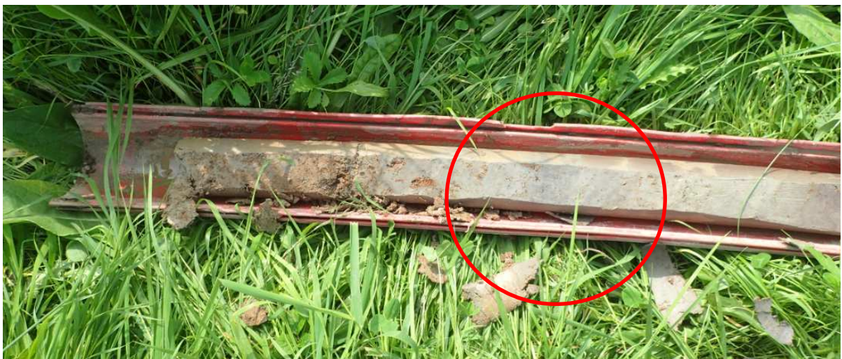
Laklaag in boring 6.
