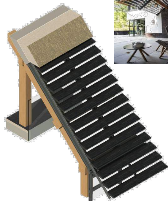
IMPRESSIE LAMELLEN IN DAK
