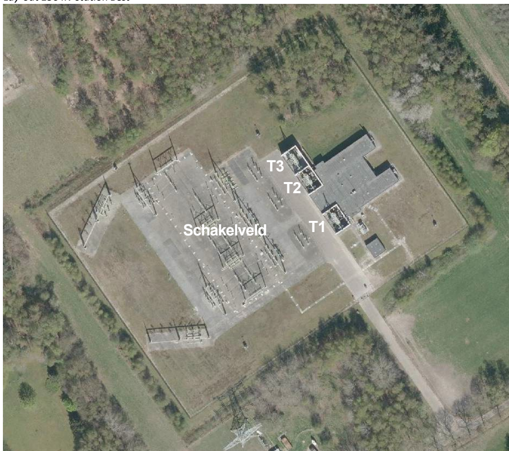
f2.1 Lay-out 150 kV station Best
