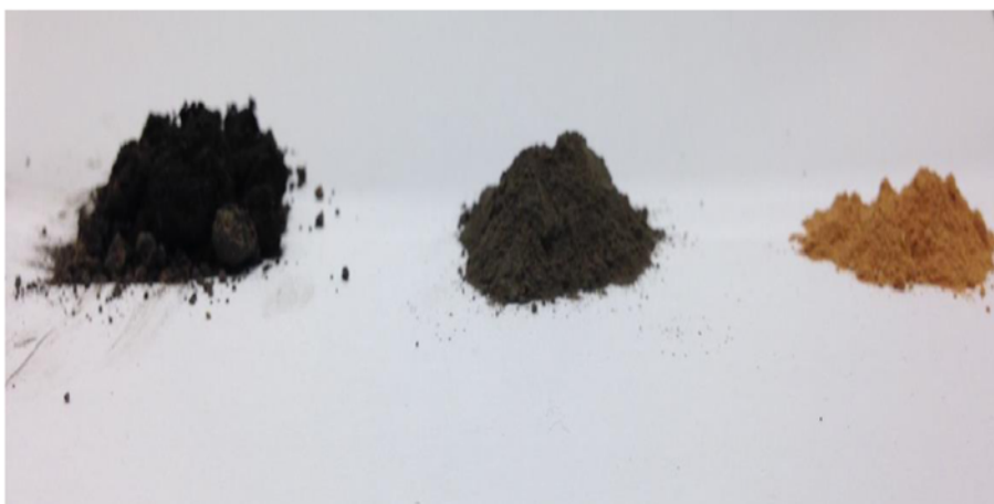
Figure 3. The different stages of the sample: left the as-received sample; middle the dried and milled sample; right the milled sample after air heat treatment at 800°C.
