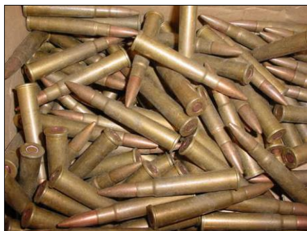
Klein Kaliber Munitie (KKM), kaliber .303
