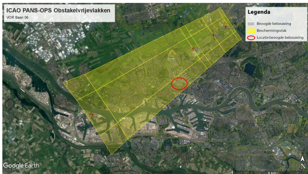
Figuur 7.8: VOR RWY06 – Protection surface overview
