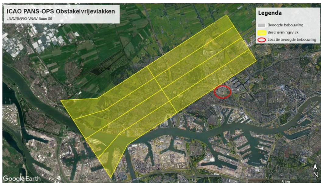
Figuur 7.14: RNP RWY06 LNAV-VNAV – Protection surface overview
