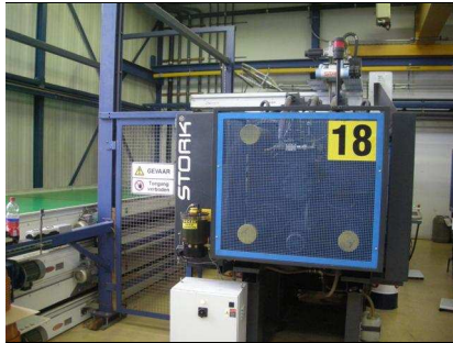
Figure 2.12 Proper fencing of an injection moulding machine
