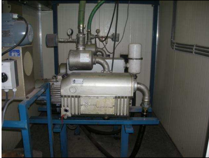
Figure 2.8 Vacuum installation for transporting granules
