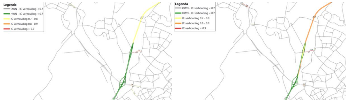
Figuur 3-3: I/C plot, 2030 autonoom (links: ochtendspits, rechts: avondspits)
