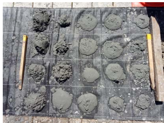
18. B-04 Boorlaag 10 – 15m – mv
