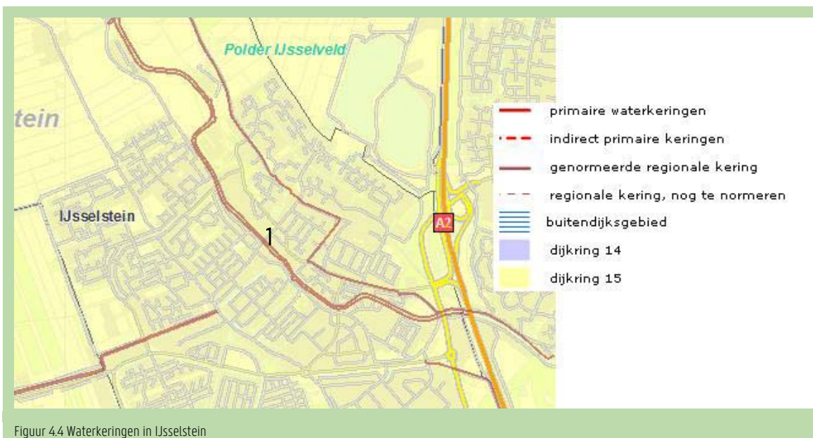
Figuur 4.4 Waterkeringen in IJsselstein
