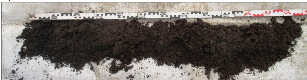
Profielboring in beplantingsstrook.
