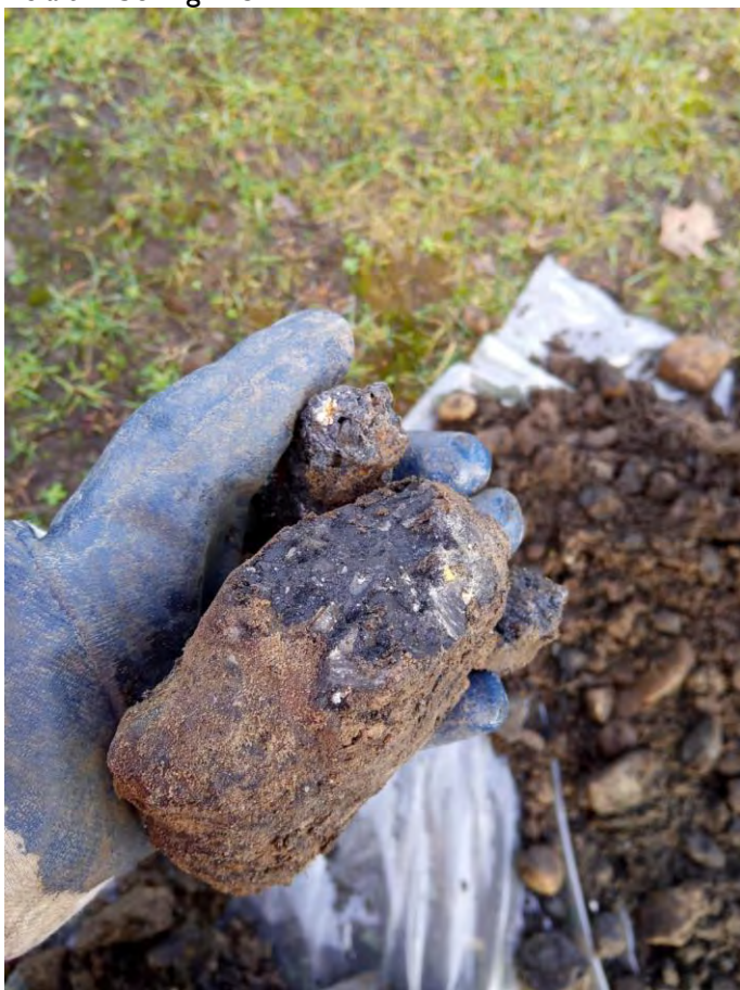
Asfalt in boring 225
