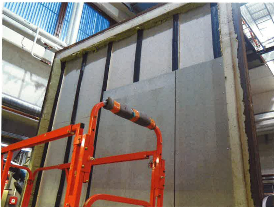
Figure 2. Fixing the façade boards on the exposed side
