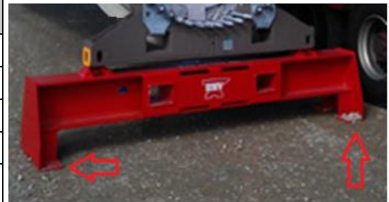
Figure 30: Example of component bracket. Arrows are showing the foot print area.
