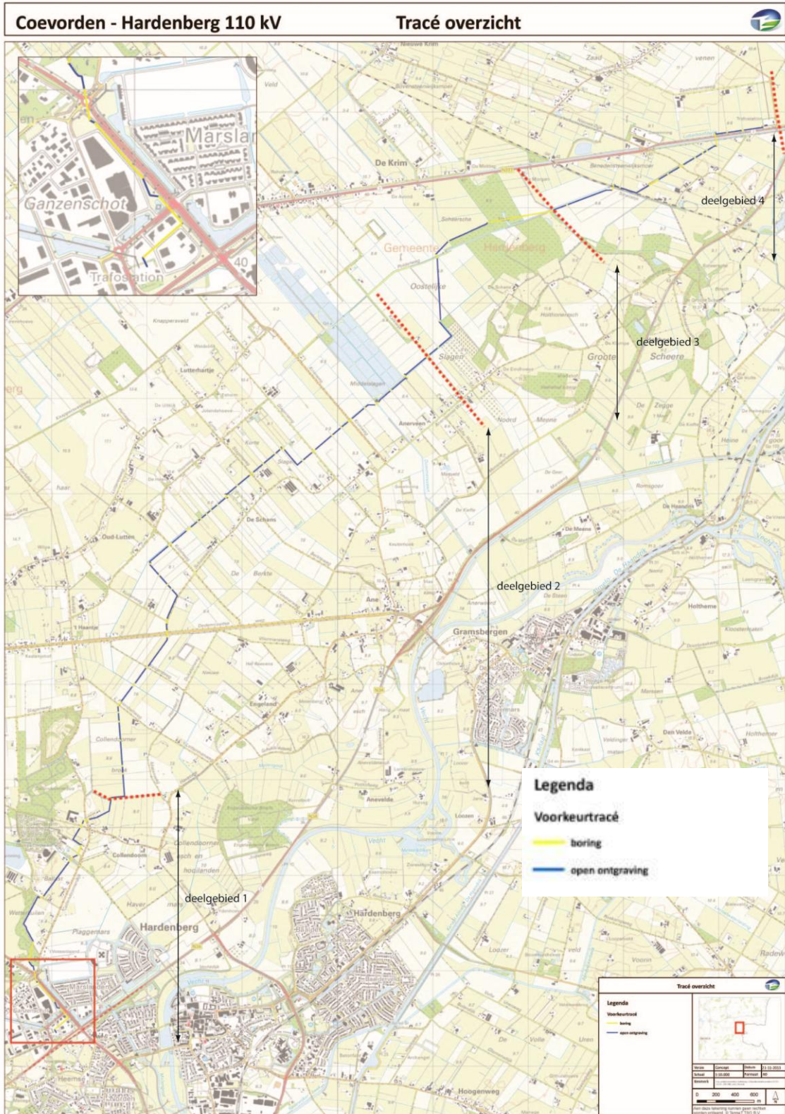
Figuur 5 tracé Coevorden – Hardenberg (geel = boring, blauw = open ontgraving)
