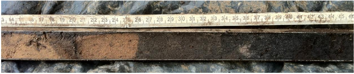
Boring 5: Top dekzand.
