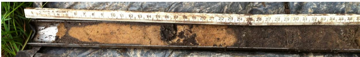
Boring 2: Top dekzand.
