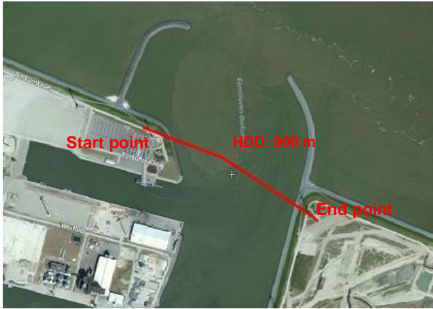
Figure 17: HDD drilling route (red line) Doekgat (Eemshaven)
