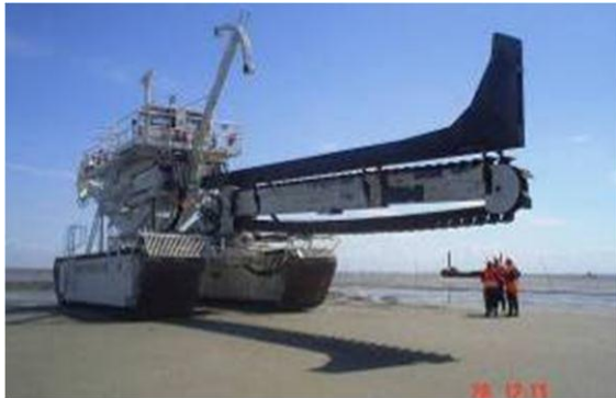
Figure 22: Typical self-supporting cable trencher
