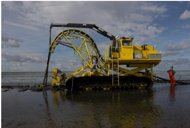
Figure 23: Typical self-supporting vibration plough
