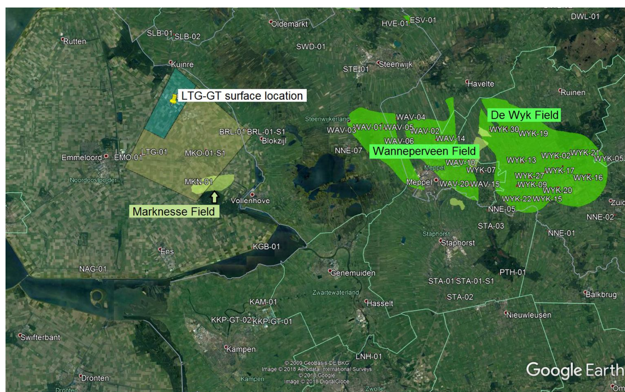
Fig. 1: Location map of the study area. The map shows local exploration wells, the exploration license areas Luttelgeest I (light blue) and Luttelgeest II (yellowish), local gas fields and the surface location of the geothermal triplet.
