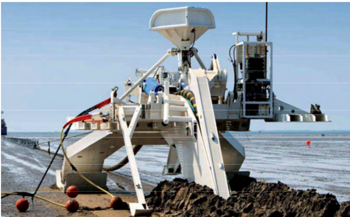
Figure 42 Sea Stallion cable plough
