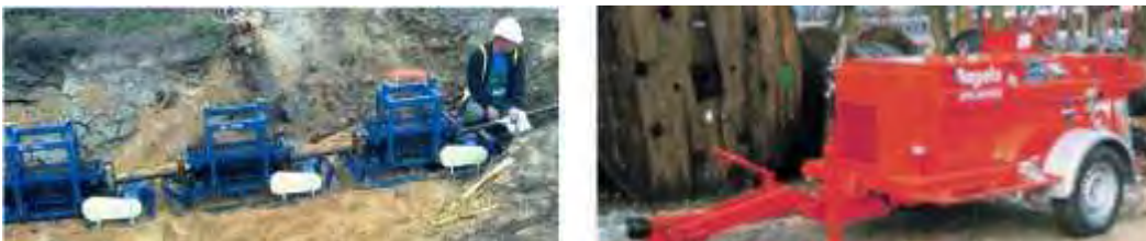
Figure 17 Typical cable tensioners (left) & cable winch (right)
