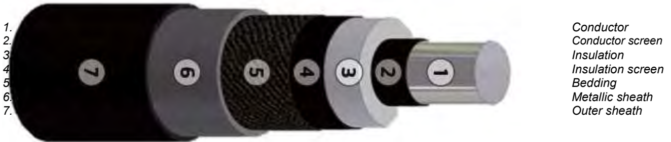
Figure 6 Typical HVAC 220 kV land export cable
