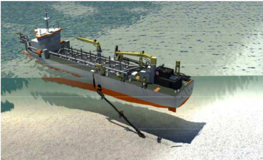
Figure 52 Trailing Suction Hopper Dredger
