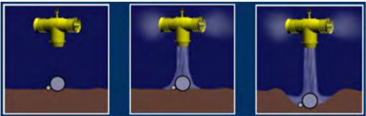
Figure 43 Mass flow excavation
