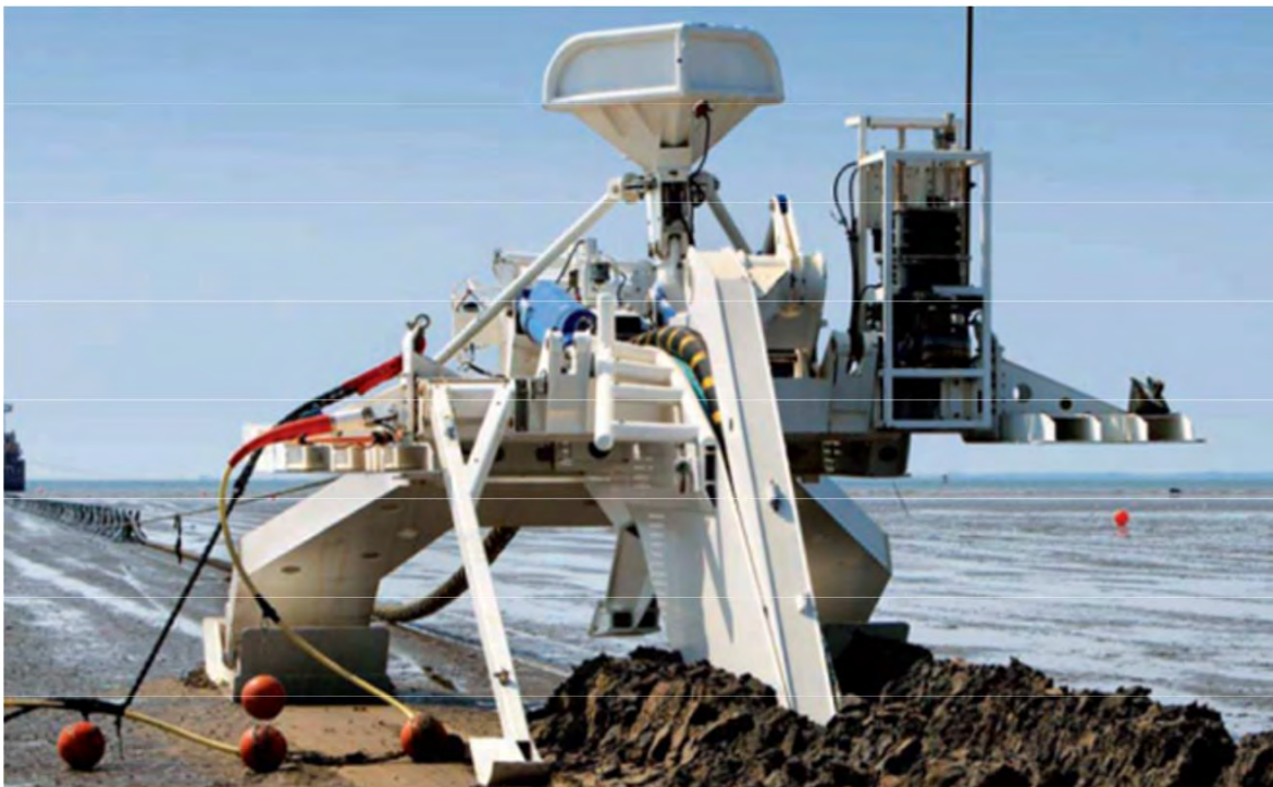
Figure 42 Sea Stallion cable plough
