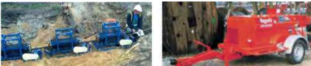
Figure 17 Typical cable tensioners (left) & cable winch (right)
