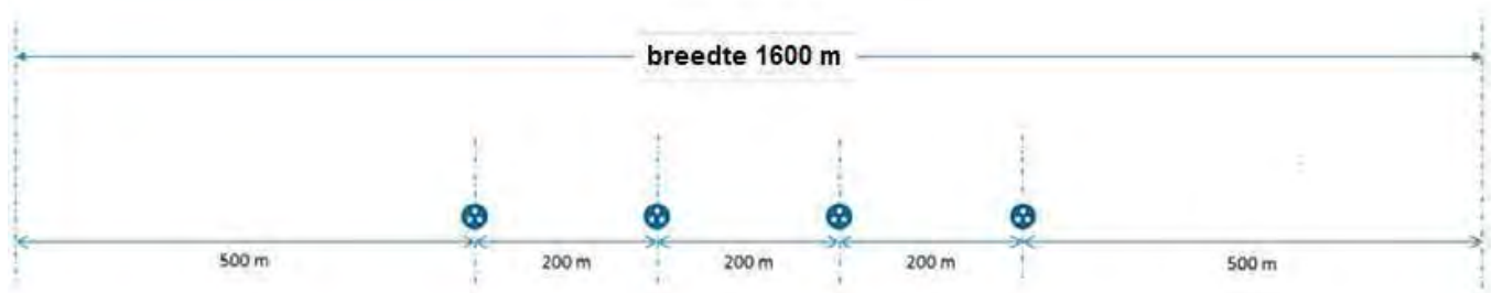
Figure 33 Cable corridor offshore section - 4 cable systems
