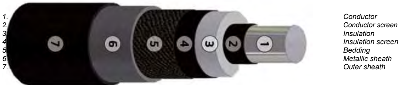
Figure 6 Typical HVAC 220 kV land export cable
