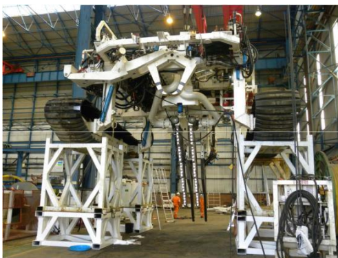
Figure 39 Typical ROV Jet trencher
