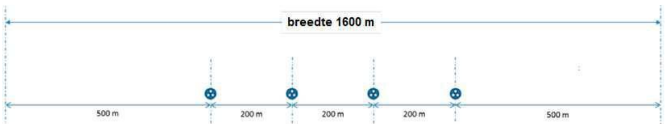
Figure 33 Cable corridor offshore section - 4 cable systems
