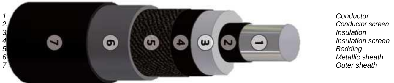
Figure 6 Typical HVAC 220 kV land export cable
