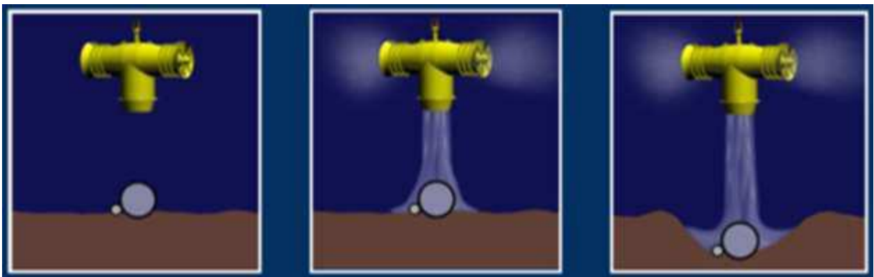
Figure 43 Mass flow excavation
